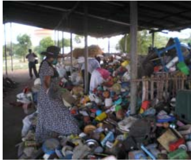
Photo 7 Manual segregation in Hambantota
